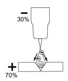
The DC power source uses what is known as DC (direct current) in which the main electrical component, known as electrons, flow in only one direction from the negative terminal (-) to the positive terminal (+). In the DC electrical circuit there is an electrical principle at work which provides that, in a DC circuit, 70% of the energy (heat) is always on the positive side. This is important because it determines what terminal to connect the TIG torch.
