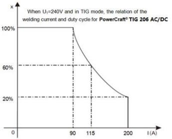
protection sensing will cut the output and the error code will displayed on the front screen. In that case, cease welding for 10~15 minutes to allow cool down with the fan running. The welding output current or the duty cycle should be reduced to allow correct operation.
