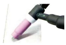
(13) Lay the outside edge of the cup on work piece with the tungsten Electrode 1~2mm from the work piece. Press and hold the trigger button on TIG torch to start the gas flow.
