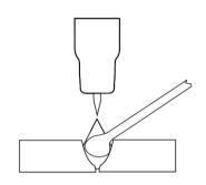
It is necessary in many situations with TIG welding to add a filler wire into the weld pool to build up weld reinforcement and create a strong weld. Once the arc is started the torch tungsten is held in place until a weld pool is created, a circular movement of the tungsten will assist is creating a weld pool of the desired size. Once the weld pool is established tilt the torch at about a 75° angle and move smoothly and evenly along the joint. The
