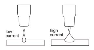
The intensity of the arc is proportional to the current that flows from the tungsten. The welder regulates the welding current to adjust the power of the arc. Typically thin material requires a less powerful arc with less heat to melt the material so less current (amps) is required, thicker material requires a more powerful arc
