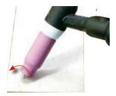
(14) With a small movement rotate the gas cup forward so that the tungsten electrode touches the work piece.
