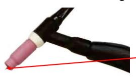
(12) Assemble front end parts of the TIG torch, fitting a sharpened tungsten suitable for the material to be welded.
