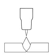
Manual TIG welding is often considered the most difficult of all the welding processes. Because the welder must maintain a short arc length, great care and skill are required to prevent contact between the electrode and the workpiece. Similar to Oxygen/Acetylene torch welding, TIG welding normally requires two hands and in most instances requires the welder to manually feed a filler wire into the weld pool with one hand while
