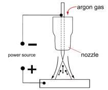
as hot as 19,000°C. It is a very pure and concentrated arc which provides the controlled melting of most metals into a weld pool. TIG welding offers the user the greatest amount of flexibility to weld the widest range of materials, thickness and profiles. DC TIG welding is also the cleanest weld with no sparks or spatter.
