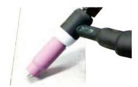
(13) Lay the outside edge of the cup on work piece with the tungsten Electrode
