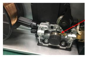
(8) Feed wire over drive roll into outlet guide wire tube, push wire through approximately 150mm
