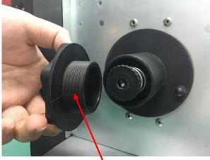
(1) Remove the spool retaining nut.
