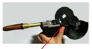
(8) Remove the spool cover by pressing button and lifting off the cover.
