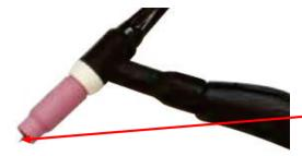
(12) Assemble front end parts of the TIG torch, fitting a sharpened tungsten suitable for the material to be welded.
